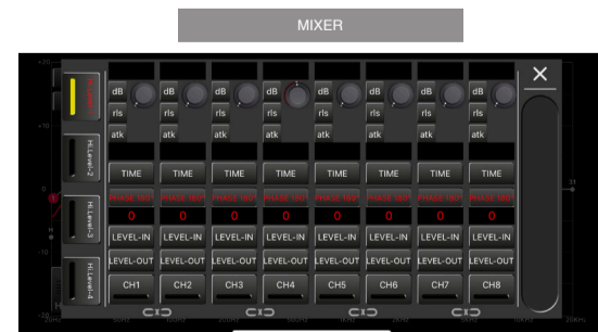
Mixer allows any input channel to be mapped to any output channel. Especially useful when you need the full 10 channel output from a stereo source such as a phone.
