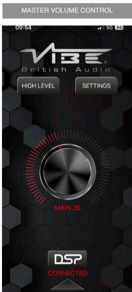
Controls the master volume for all channels from the home page of the DSP amps
